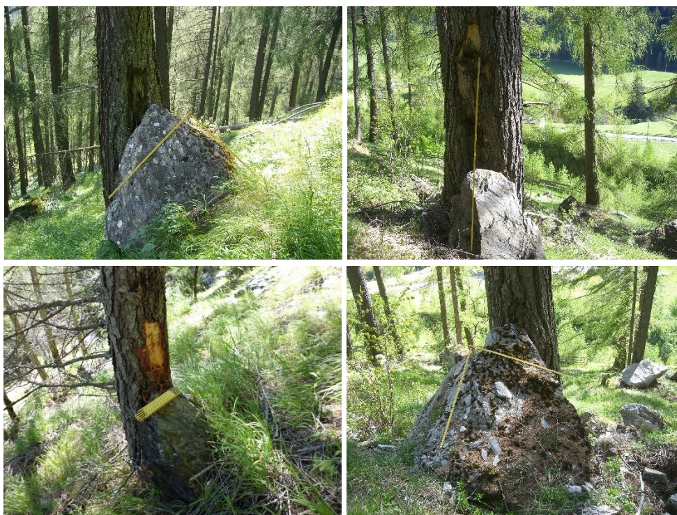
Fig.1: Impact marks and stopped blocks by rockfall protection forest (©Plörer)
